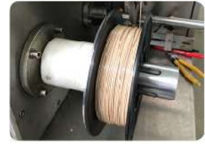
PEEK 3D打印线材挤出线 PEEK 3D printed filament extrusion production line
