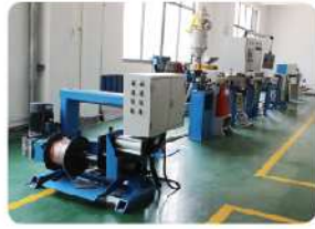
PEEK线缆挤出生产线 PEEK Cable production line
